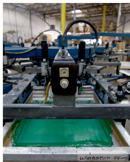
Close up of one of Promo Ink's M&R screen printing machines.
